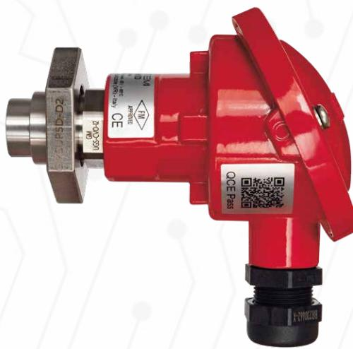
The GMSC245D-FM is a spark detector for aspiration plants' ducts. In these systems, the sparks exist in the form of small hot bodies caused by the production process (machine tools, etc...) which pass through the air flow in ducts; they mostly emit infrared radiation that are picked up by our detector's sensor. It can also detect high speed hot bodies up to 36 m/s.
