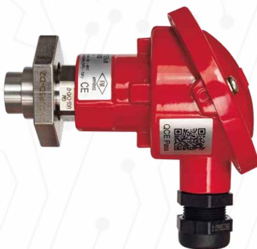
*The GMSC245D-FM is a Sparks Detector for the pipelines in a dust suction systems (dust collectors), and pneumatic transport of the dusts. In that plants, the sparks are small bodies, very hot or incandescent, generated by processing (machine tools, etc..) that transit in the ducts, these sparks emit radiation in a field of frequencies predominantly in the infrared.*
